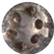
Injector after one P.i. treatment.
