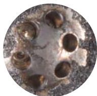
Injector after one P.i. treatment.
